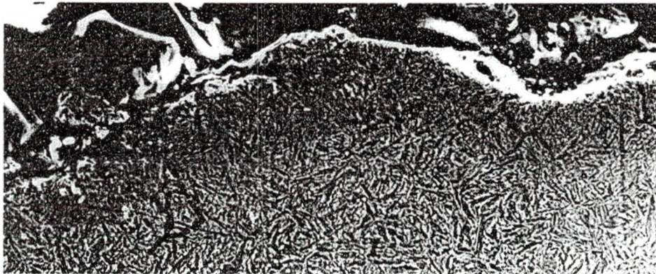
Figure 56 Decarburized Layer of AISI 8620 Test Cylinder at a Magnification of 1000
